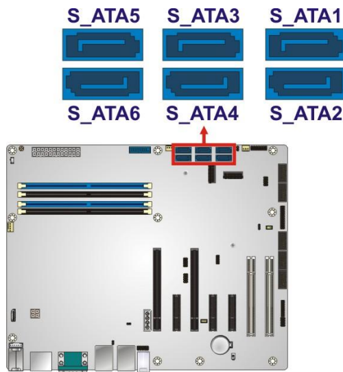
Figure 3-24: SATA 6Gb/s Drive Connector Locations
