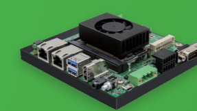
NVIDIA Developer Kit - Supports Jetson Orin NX / Nano - 5G, 4G, Wi-Fi - 4 × USB 3.0, 2 × LAN
